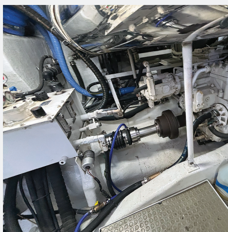
PSS Pro Shaft Seal installed on M/Y Silver Mama
