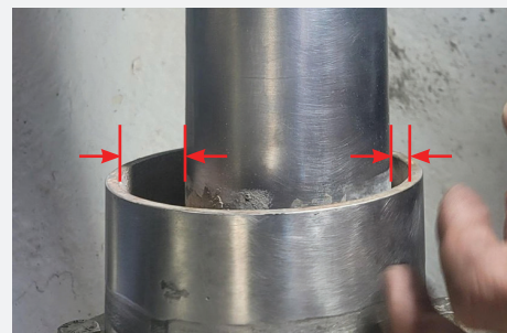
Propeller shaft off-center within the stern tube.
