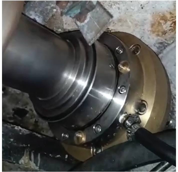
PSS / AES Seal #AZT5471923712014A with PSS Mounting Flange #07-F11-0AES.
